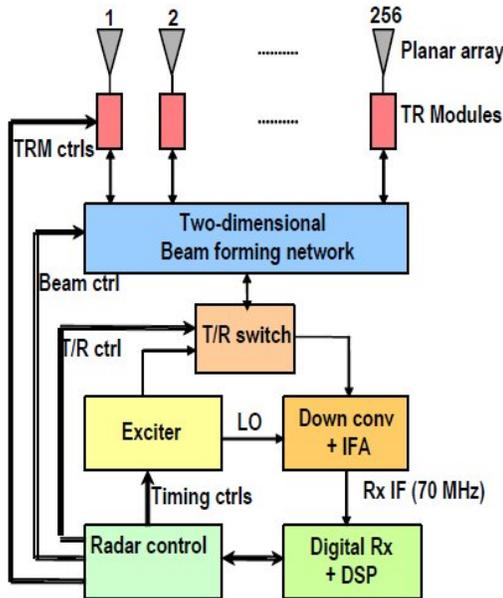
Figure 2. Block diagram of the UHF Wind Profiling Radar
