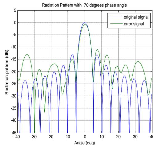
Figure 5: Effect of random error with 70<sup>0</sup> phase angle
